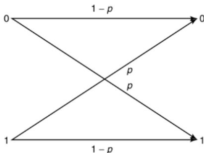
FIGURE 7.5. Binary symmetric channel.  $C = 1 - H(p)$  bits.
